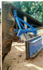
SCRAPER FITTED TO TRACTOR FOR EASY USE ON CATTLE FARM
