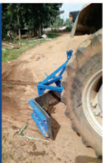
SCRAPER FITTED TO TRACTOR FOR EASY USE ON CATTLE FARM
