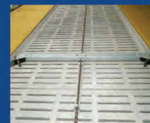
Grid Scraper Galvanised version with rubber rotors
