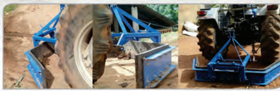
Scraper Fitted To Tractor For Easy Use On Cattle Farm
